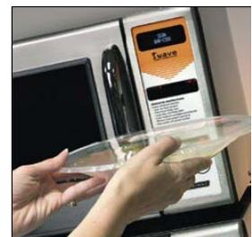
**C-Press** As directed by the LED display, the operator presses the large start button. A countdown display indicates the time remaining.
