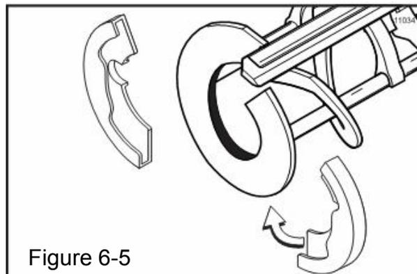
Slide the beater assembly the rest of the way into the freezing cylinder. Make sure the beater assembly is in position over the drive shaft. Turn the beater slightly to be certain that the beater is properly seated. When in position, the beater **will not** protrude beyond the front of the freezing cylinder.
