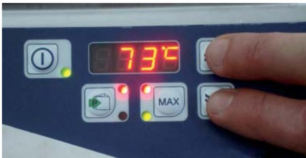
You can check the temperature of the fry top at any time by pressing the keys
